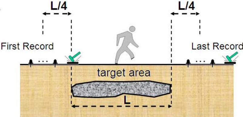
The increment of the receiver array and shot point is called source-receiver move ( $dSR$ ) (see diagram below) and influences lateral resolution of the survey: the smaller, the higher resolution. However, the higher resolution results in a higher overall cost as the survey will take more time and end up with more data. The following criteria can be used:  **$dSR = 1dx$  (highest)**,  **$(2-4)dx$  (good)**,  **$(4-8)dx$  (fair)**,  **$(8-12)dx$  (minimum resolution)**.
